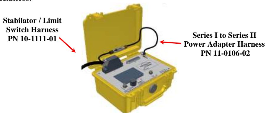
Figure 3-2 – Power Hook-up with Series I UxValidator
