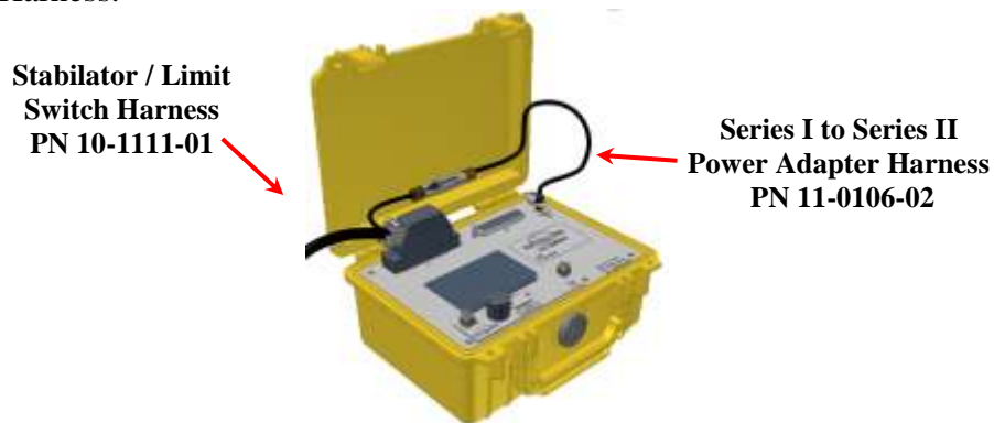
Figure 2-2 – Power Hook-up with Series I UxValidator
