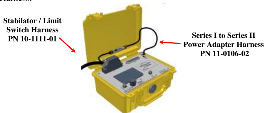
Figure 4-2 – Power Hook-up with Series I UxValidator
